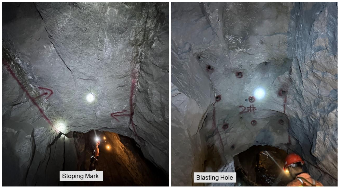
Figure 16.8: Stoping Management and Blasting Holes
