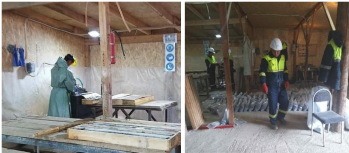
Figure 10.3: Core cutting and sample preparation in the core logging facility at the project site.
