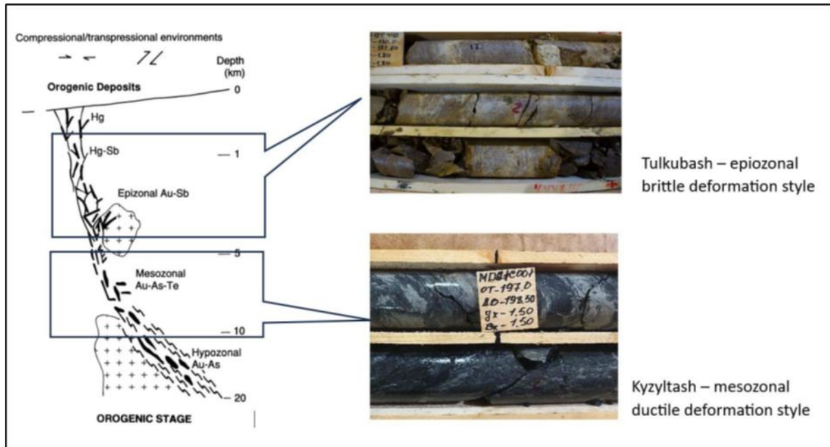
Figure 7.4: Scheme of the orogenic gold deposit as a function of depth in the crust (Groves et al., 1998), with modifications.
