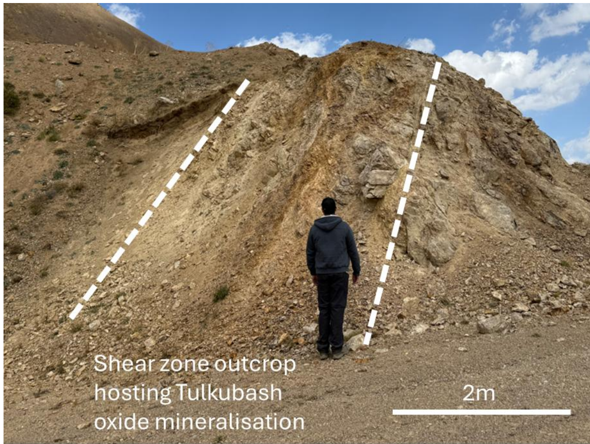
Figure 8.1: Zone of structurally hosted oxidation and alteration within the Tulkubash deposit.
