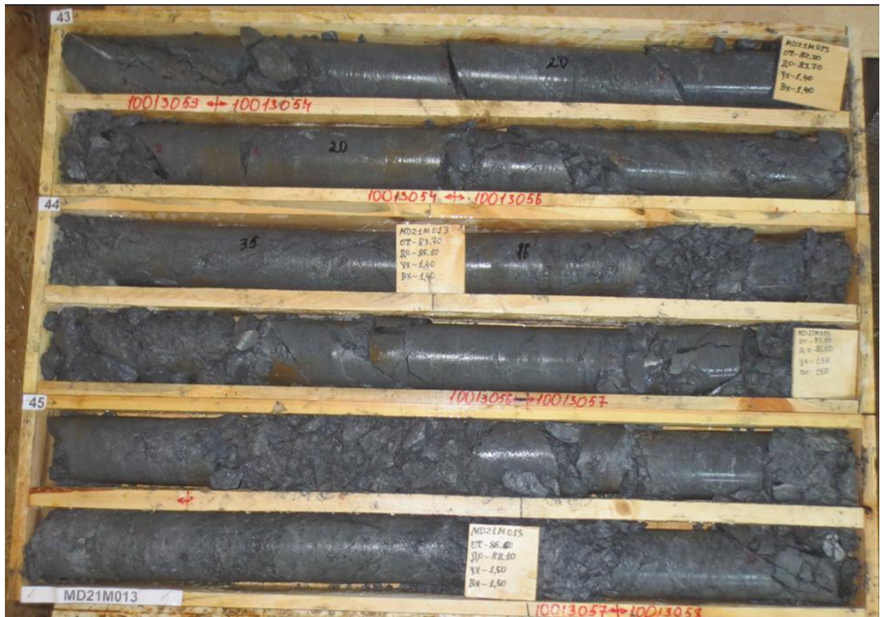
Figure 8.2: MD21M013 – Intensive sulfidation with quartz veining and brecciation of a mineralised intercept hosted in the Kyzyltash Main zone.
