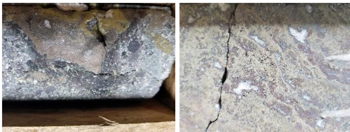
Figure 7.4: Massive Sulphide Zone with Zinc-rich Mineralization
