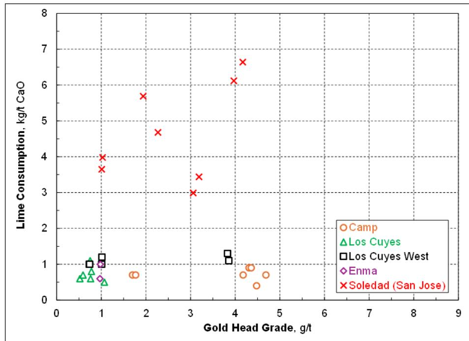
The consumption of lime (CaO) is presented in Figure 13-4 as a function of gold head grade. Average values are 0.7 kg/t for the Camp domain, 0.7 kg/t for the Los Cuyes domain, 1.1 kg/t for the Los Cuyes West domain, 0.8 kg/t for the Enma domain and 4.6 kg/t for the Soledad (San Jose) domain.
