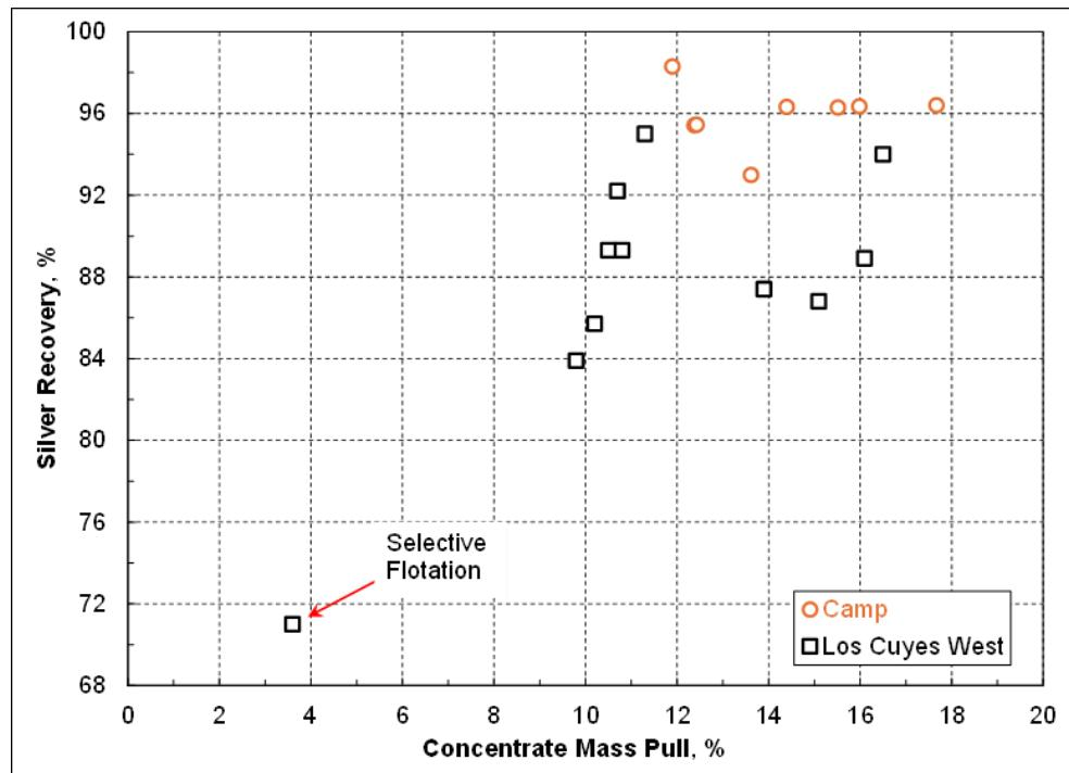
**Figure 13-15: Relationship between Silver Recovery and Silver Head Grade from the Flotation of Feed Samples and Gravity Tail Samples**
