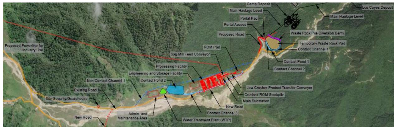
Channels and ponds are designed to convey or contain the 1:100 year, 24 hour precipitation event. Local unit costs for construction were used when available. In the absence of local rates, rates for Canadian projects were used.
