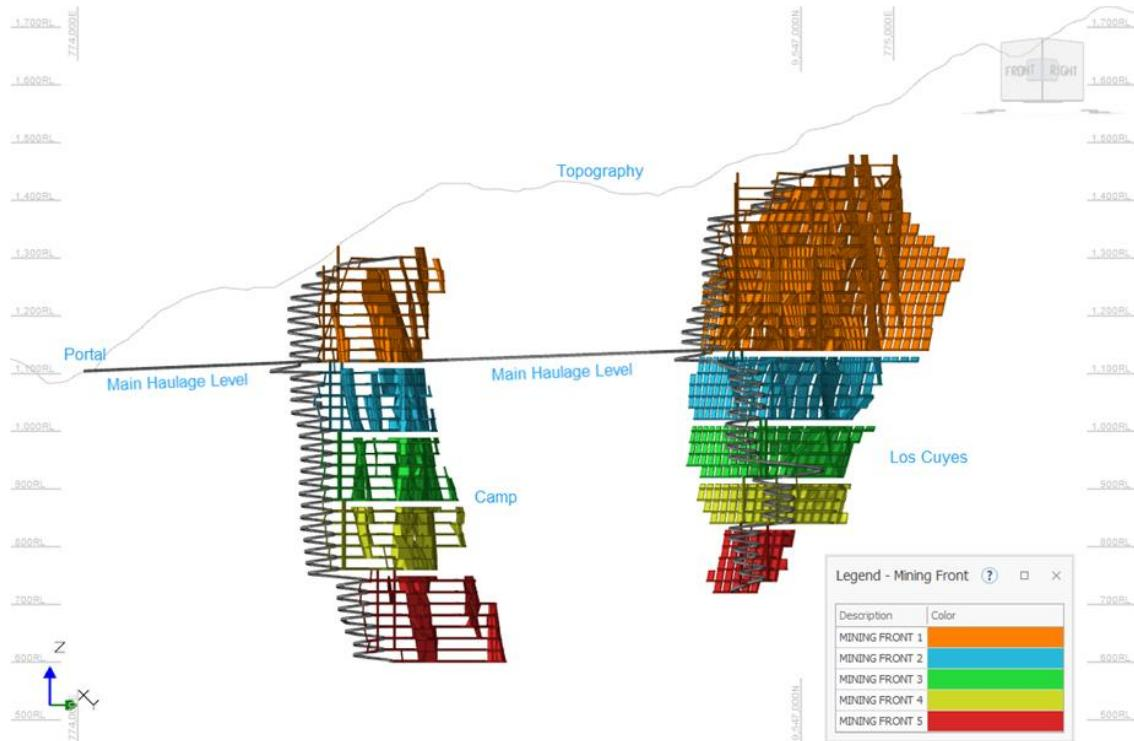
**Figure 16-13: Condor Underground Mine Layout Showing Mining Method (Top-Front Orientation)**
