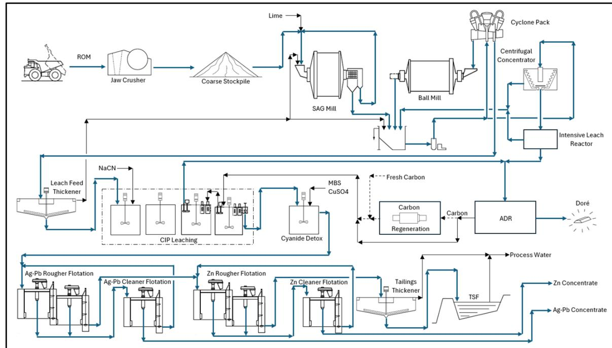
**Figure 17-2: Mill Layout – Overall Mill Site**
