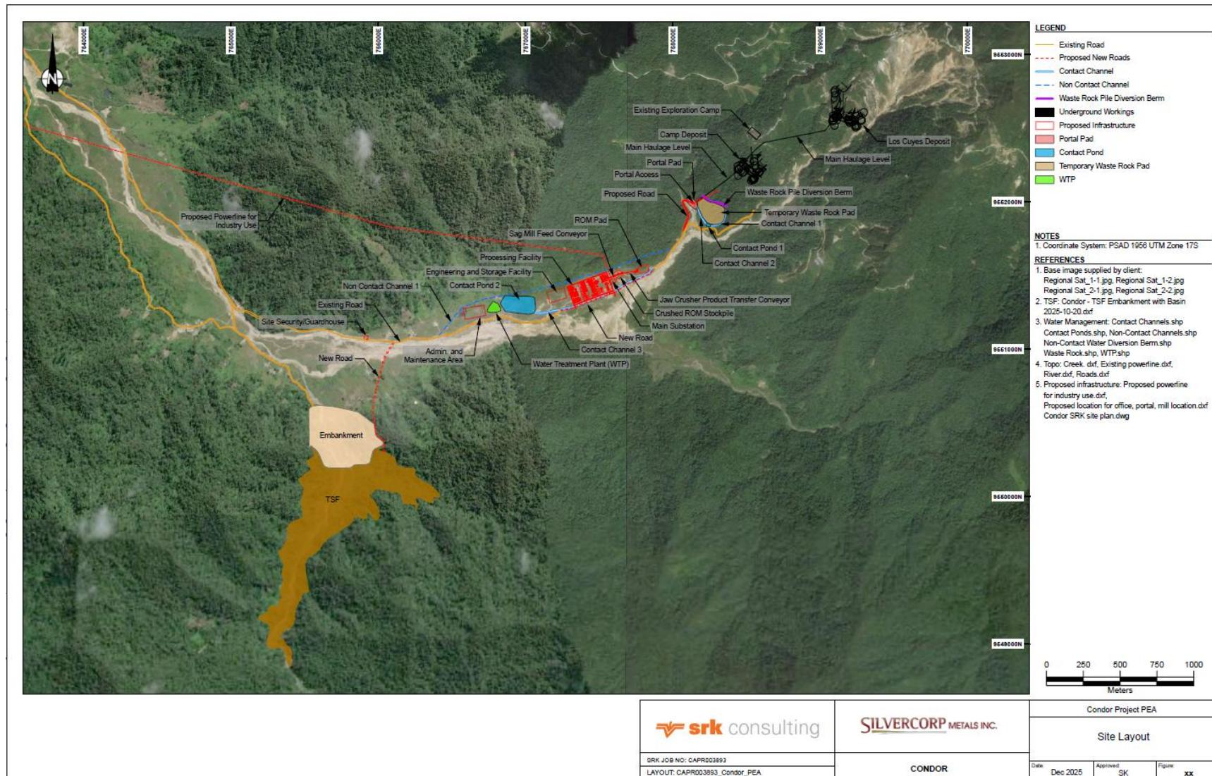
Seepage from the embankment will be captured in a seepage collection pond near the downstream toe of the embankment. The seepage collection pond will also intercept sediment runoff.
